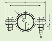
Fluorocarton coated or galvanised with neoprene isolating pad
